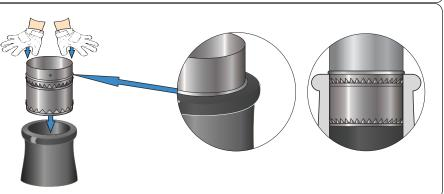
3. Reattach the cowl to the barbed section using the original screws.
